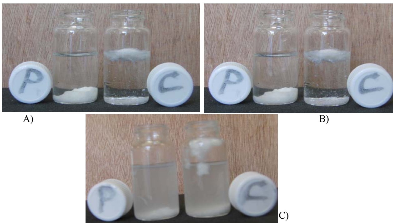
Figure 1. Water suspending of medicine material. SEROQUEL XR, powders before and after the plasma treatment. A) after 1 min, B) after 5 min C) after 10min
